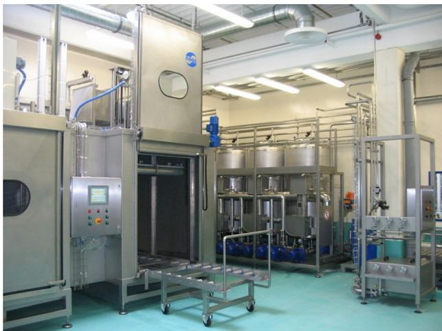
and high performance in-line cleaning systems in modular variations. Multi-stage filtration, dirt extraction belts, machine self-cleaning with CIP programs are the basic features of our technology.
